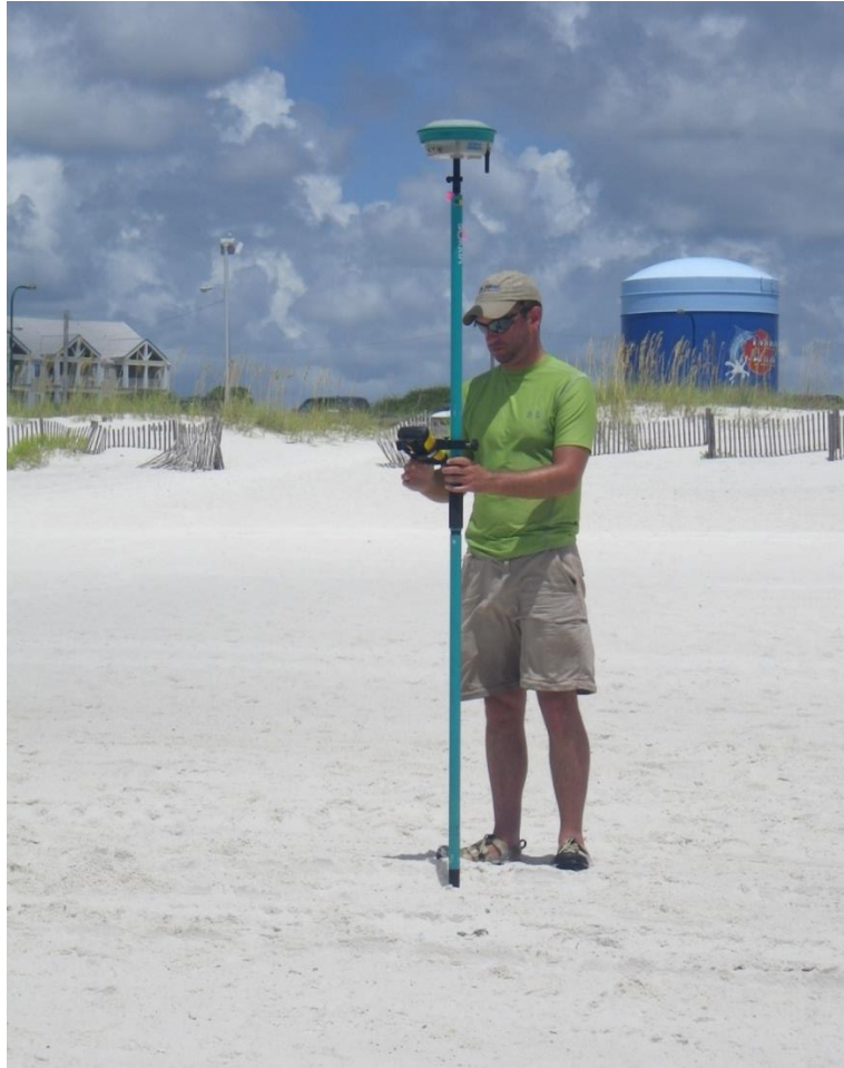
Figure 4.1 GPS Satellite Survey Equipment
